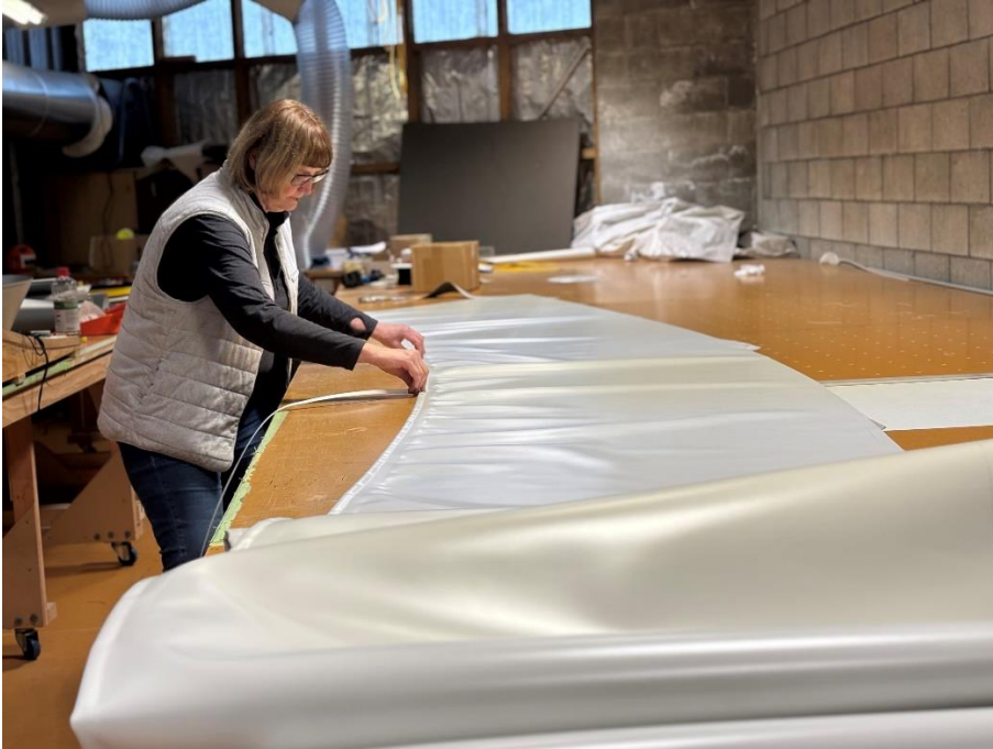
Josee Derden, Collar Manufacturing Manager, providing quality assurance of the seam on a lower portion of a Naiad collar before continuing fabrication at KJL Sails, Picton New Zealand.
