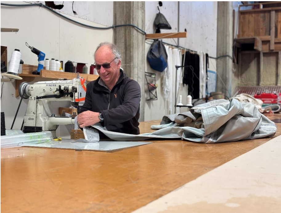
Bill Richards, Textile Fabricator, sewing a repair for a yacht Bimini at KJL Sails, Picton New Zealand.
